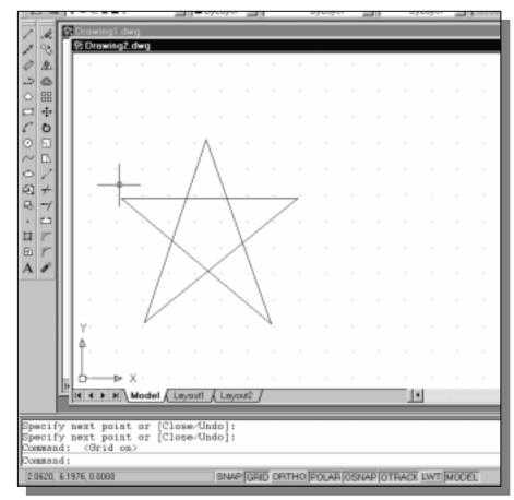
The GRID option creates a pattern of dots that extends over an area on the screen. Using the grid is similar to placing a sheet of grid paper under a drawing. The grid helps you align objects and visualize the distance between them. The grid is not displayed in the plotted drawing. The default grid spacing, which means the distance in between two dots on the screen, is 0.5 inches. We can see that the sketched horizontal line in the above sketch is about 3.5 inches long.
