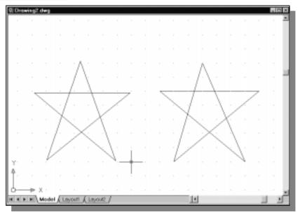
6. In the command prompt area, notice that "*Command:*" is displayed. This indicates that AutoCAD is waiting for us to activate the next desired command.
