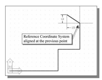
11. Using the *relative rectangular coordinates entry method* to create the next line, we can imagine a *reference coordinate system* aligned at the previous point. Coordinates are measured along the two reference axes.
