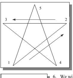
5. We will create a freehand sketch of a fivepoint star using the *Line* command. We will create the sketch near the center of the drawing window. Do not be overly concerned with the actual size or the accuracy of your freehand sketch. This exercise is to give you a feel for the **AutoCAD<sup>®</sup> 2002** user interface.
