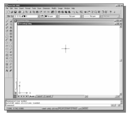
Note that two graphics windows, *Drawing1* and *Drawing2*, are opened. AutoCAD automatically assigns generic names, *Drawing X*, as new drawings are created. In our example, AutoCAD opened the first graphics window (*Drawing1*), using the default system units. The second graphics window (*Drawing2*) was opened when we chose to create a new drawing from scratch using the default English units.
