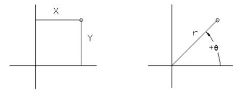
For planar geometry, the polar coordinate system is very useful for certain applications. In the polar coordinate system, points are defined in terms of a radial distance, r, from the origin and an angle  $\theta$  between the direction of r and the positive X axis. The default system for measuring angles in **AutoCAD**<sup>®</sup> 2002 defines positive angular values as counter-clockwise from the positive X-axis.
